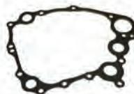
R&D's new Front Cover Gasket features a metal reinforced center that enables it to be reusable when servicing the supercharger clutch.
