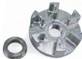
Billet aluminum drive coupler for the Kawasaki 900/1100 that uses the 750/800 damper. This coupler is for putting a 900/1100 engine into a
