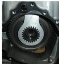
This R&D tool enables the clutch to be changed in a matter of only minutes. With the supercharger and front engine cover removed the tool drops down through the case and secures the drive gear at the front of the crankshaft from rotating when the clutch is removed and installed. This is a "must have" tool that will save massive amounts of time for any mechanic.
