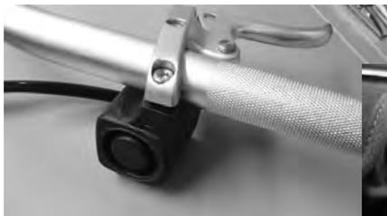
JP7043/JP7044 can be installed with Hot Products Throttle Lever 58-0970 & 58-0971 as pictured above.
