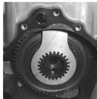
This R&D tool enables the clutch to be changed in a matter of only minutes. With the supercharger and front engine cover removed the tool drops down through the case and secures the drive gear at the front of the crankshaft from rotating when the clutch is removed and installed. This is a "must have" tool that will save
