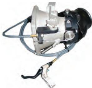
Easy-Trim System was designed to allow riders of all levels to get a fair amount of trim with a light pull on the lever. The system will give you 30-35 degrees of trim. The system is constructed of anodized billet aluminum for strength and light weight. It can
