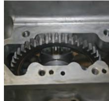
The R&D Super Clutch Drive Gear System is CNC machined from premium billet steel alloy, heat treated for Bionic strength and hardness, precision ground to strict aircraft tolerances, and polished for a low friction finish.
