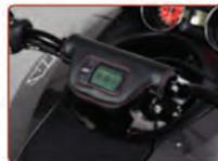
USB port. GPS Track mapping function displays "live" lap times and related functions for buoy course training purposes. Features LED warning lights to notify operator of major engine concerns.
