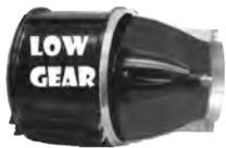
In low gear the shuttle lets a large volume of water be moved to accelerate the craft.
