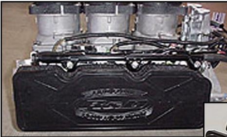
GP 1300R Power Plenum
