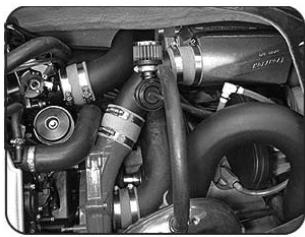
Power Cooler Kit with Performance Blow-off Valve
