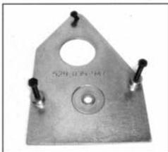
**Support Plate 4-TEC Supercharged Engines**
